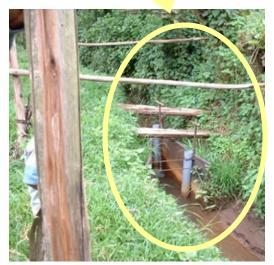
Topsoil loss from slopes upstream in the watershed (top) is assessed with a visual turbidity monitor (bottom).
